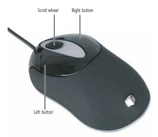
The *mouse* is a device that controls the pointer movement on the computer display. This illustration shows the standard mouse.
